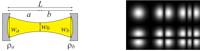
Figure 7.29: (code) (Left) Scheme of a linear cavity. (Right) Radial profiles of the lowest order transverse Hermite-Gaussian modes \text{TEM}_{mn} of a linear cavity.
